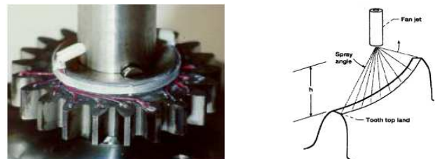
Fig. 2 Shows, previous test (left) and up jet lubrication (right).
