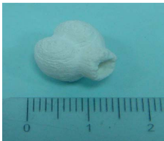
Fig. 5 The HA bone scaffold model with hollow shell structure obtained by laser curing under layers thickness of 100 \mu\text{m} , laser power of 15 W, scan velocity of 150 mm/s and a laser frequency of 10 KHz
