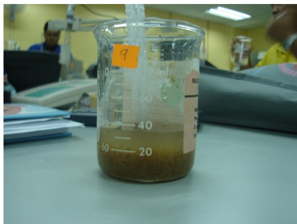
Fig. 2 Chemical treatment of corn husk
