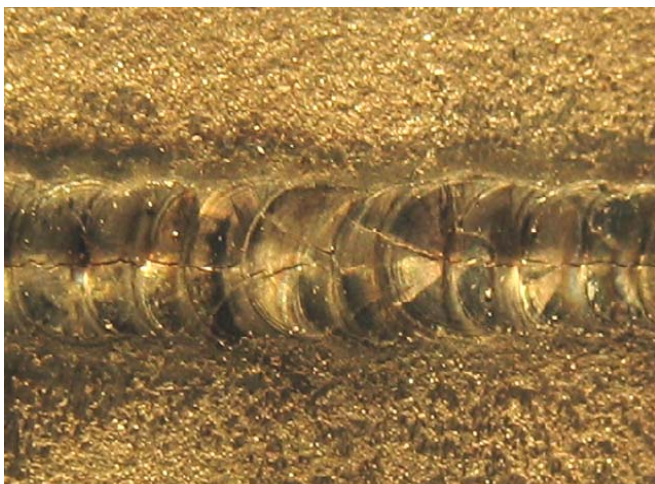
Fig. 2 Macroscopically image of a Wiron 99 alloy welded without filler material: longitudinal discontinuous crack on the weld trajectory
