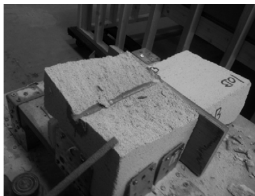
Fig. 3 Total spalling, crushing in front of reinforcement
