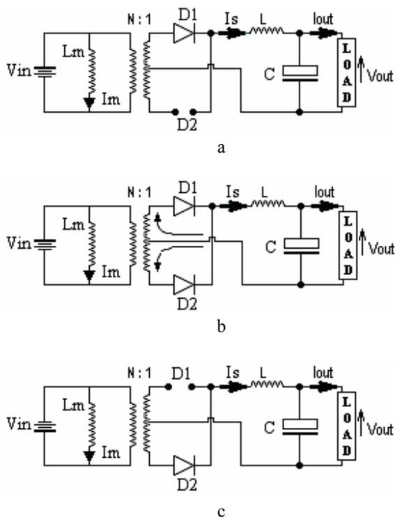
Fig. 2 Different operating modes of the converter
