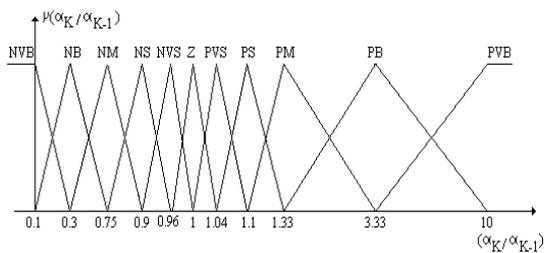
Fig. 6 Membership functions for Phase-shift angle ( $\alpha_k/\alpha_{k-1}$ )
