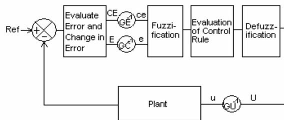
Fig. 4 Basic structure of the fuzzy controlled system
