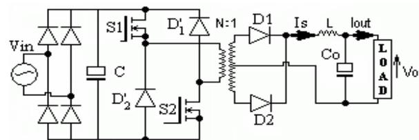
Fig. 1 Main system of arc welding machine
