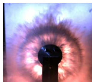
Fig. 8 The shape of liquid dispersion flow, when the detonation cord is 5 \text{ g} \cdot \text{m}^{-1} , the diameter of cylindrical film is 150mm. The liquid is the mixture of water and glycerin with capacity ratio of 5:5
