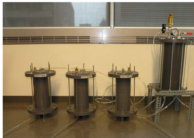
Fig. 1 Column leach test cells with pressure vessel setup
