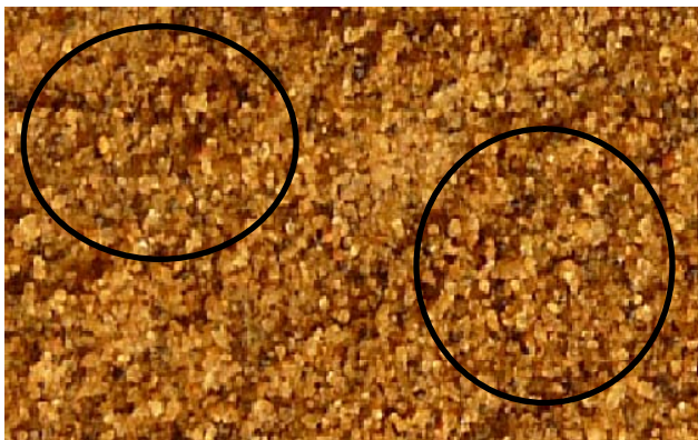
Fig. 4 Digital image for the upper surface of a 95% sand and 5% bentonite liner leached by biofuel under a pressure of 100 kPa (cracks are showed in circles)
