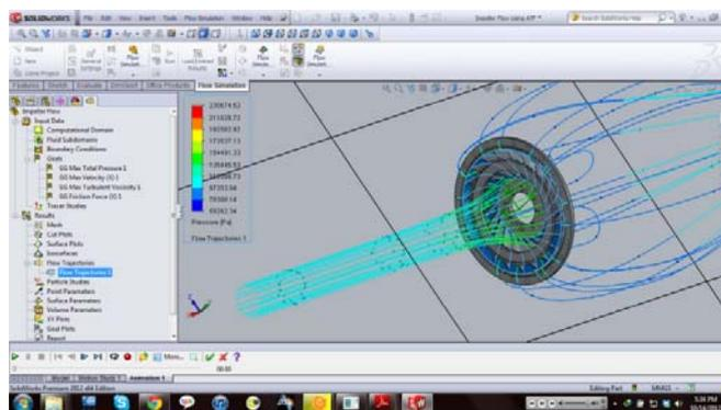
Fig. 4 Flow Trajectory of Hydraulic Fluid in Impeller
