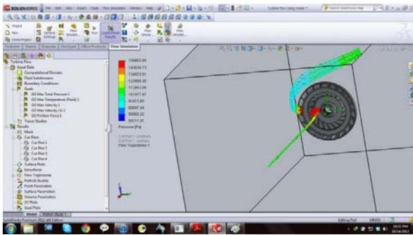
Fig. 5 Flow Trajectory of Hydraulic Fluid in Turbine
