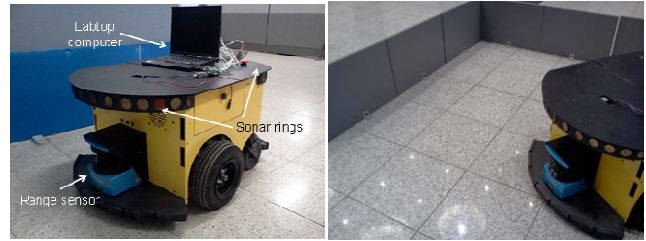
Fig. 10 Mobile robot equipped with the laptop computer, 2D laser rangefinder (left) and the environment made of the series of panel (right).
