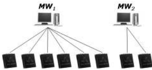
Fig. 2 RFID middlewares with the connected RFID readers
