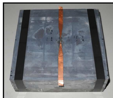
(a) Electrode arrangement for outside discharge
