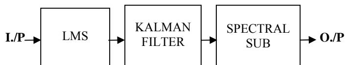
Fig. 4 Block diagram representing Cascading of LMS with Kalman filter and spectral subtraction
