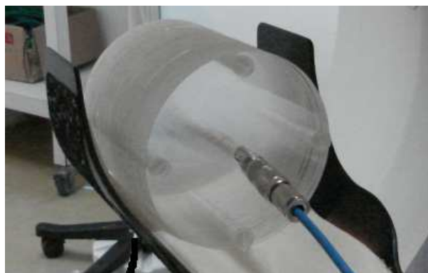
Fig. 3 Dosimetric head phantom positioned in the head support on the top of the patient couch with the detector inserted in the central hole
