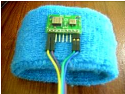
Fig. 2 Accelerometer module attached to a wrist band
