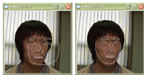
Fig. 4 Face alignment results, (a) basic AAM-based one (b) the proposed progressive AAM-based one (Domestic DB)
