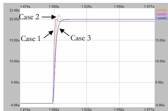
Fig. 9 Transient response of the SI cell
