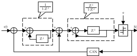
Fig. 2 Second order Sigma-Delta modulator block diagram
