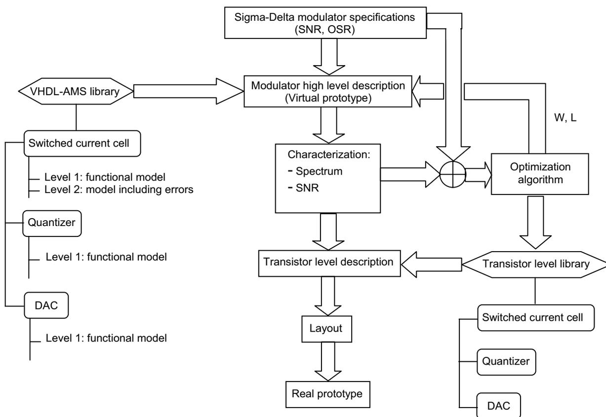
Fig. 1. Diagram of the hierarchical design flow
