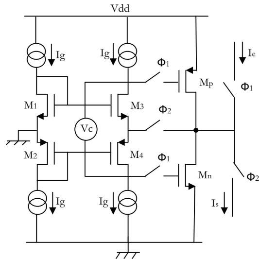
Fig. 4 Class AB switched current cell
