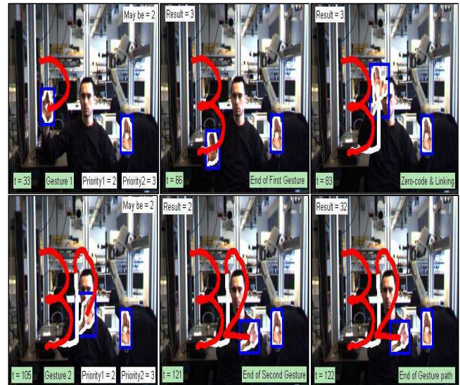
Fig. 15. System output for continuous gesture 32, where at t=66 the first gesture is ended with result 3, at t=83 the linking between two gestures, at t=121 the second gesture is ended with result 2 and at t=122 the final result is 32.
