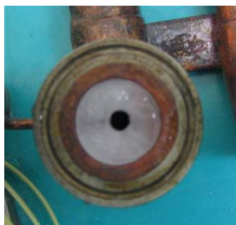
Fig. 4 A close-up of the ice layer formed
