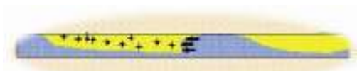
(c) A sudden phase change of water vapor trapped and creates a vacuum
