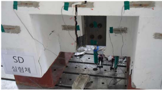
Fig. 8 Crack in SD Type
