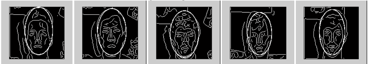
Fig. 3(e) Ellipse overlapped with edge images
