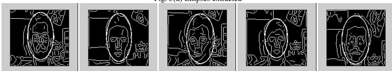
Fig. 5(e) Ellipses overlapped with edge images
