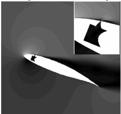
Fig. 9 Contour plots of velocity magnitude (m/s) over an airfoil at angle of attack, \alpha = 22^\circ , blowing-out segment
