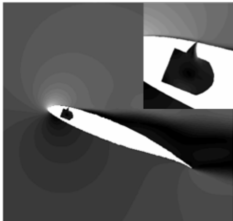
Fig. 8 Contour plots of velocity magnitude (m/s) over an airfoil at angle of attack, \alpha = 22^\circ , suction segment
