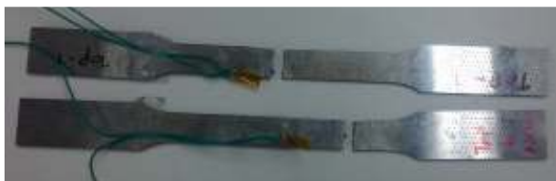
Fig. 10 Broken rail test coupons after tensile test
