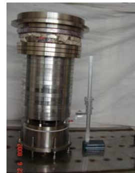
Fig. 5 Test Device of the Pulling Force Measurement
