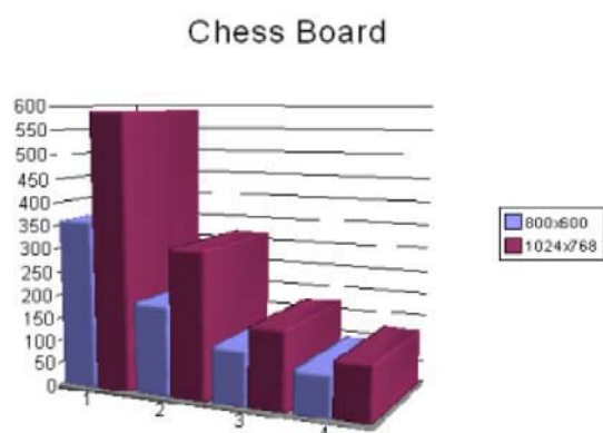
Fig. 6 Results of rendering chess.pov on a cluster with varying number of processing slave nodes
