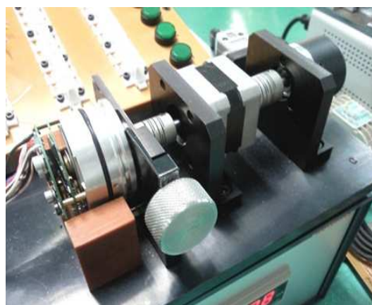
Fig. 5 Motor & encoder test equipment
