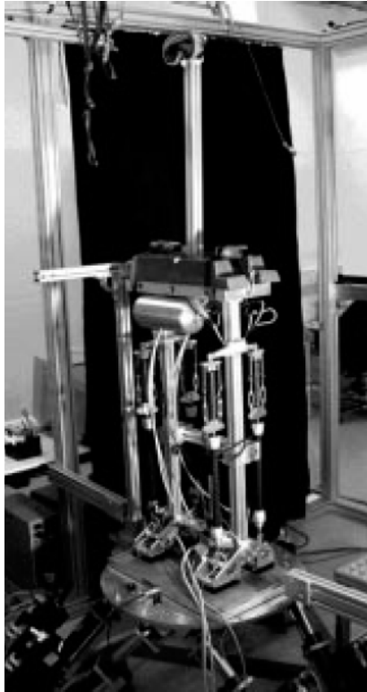
Fig. 2 Photograph of humanoid robot 'PostuRob' standing on motion platform.
