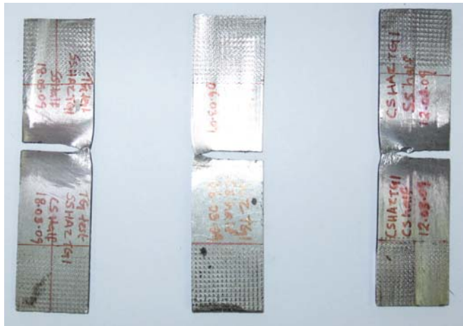
Fig. 1 FCG tested welded specimens
