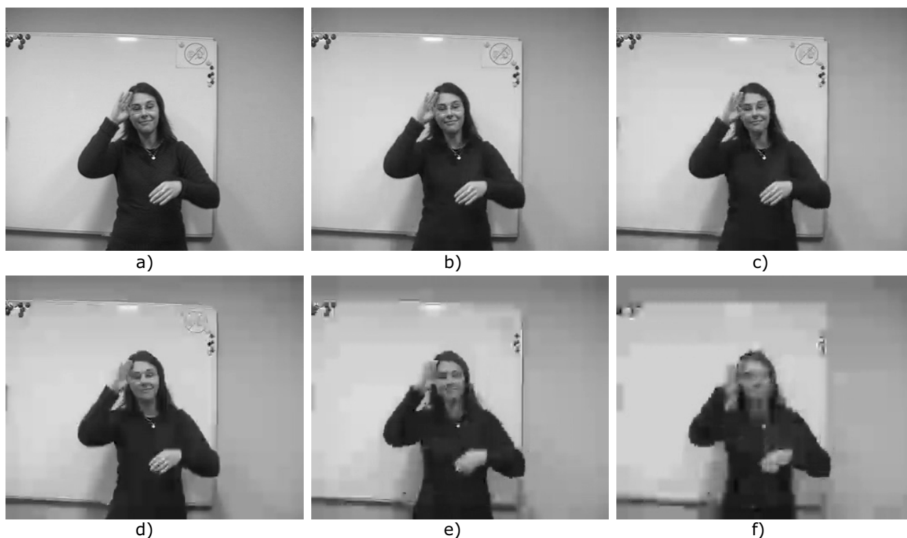
Fig. 3. 25th picture taken from the experiment: a) Original image; H.264 decoded frame with parameter: b) QP=30 c) QP=35 d) QP=40 e) QP=45 f) QP=50
