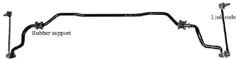
Fig. 2 The picture of the undamaged anti-roll bar analysed in this study
