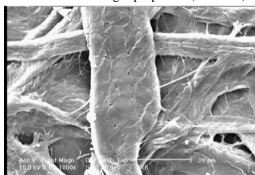
Fig. 1 SEM micrograph refined recycled fibers with magnification 1000x
