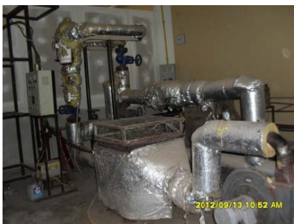
Fig. 2 The fluidized bed dryer used this study
