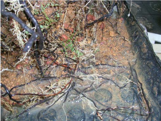
Fig. 5 Secondary roots spreading on membrane surface
