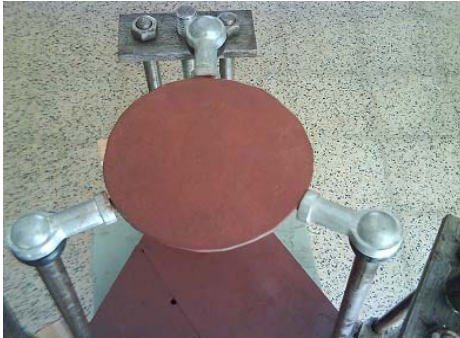
Fig. 2 A model of the 3 DOF Parallel Manipulator
