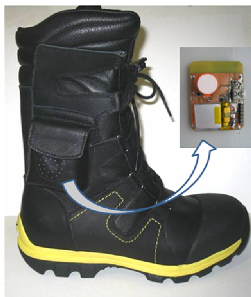
Fig. 2. Firefighter's boot with built-in pocket used for enclosing the CO 2 sensor and wireless sensing module. Right: sensor attached onto the electronic platform module
