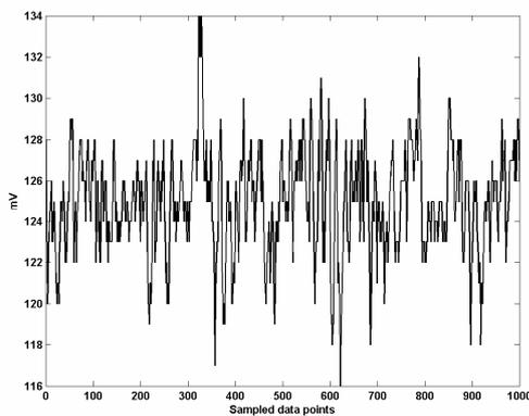
Fig. 2 Time series of recorded vibration signals-Faulty bearing
