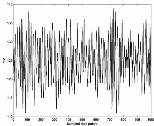
Fig. 1 Time series of recorded vibration signals-Good bearing
