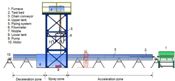
Fig. 1 Schematic of pilot scale apparatus
