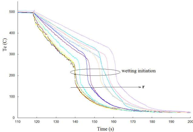
Fig. 2 Cooling curve for a water spray test ( $H=10.5in$ ,  $Q=35L/min$ ,  $T_w=25^\circ C$ ,  $T_s=500^\circ C$ ),  $r$  is distance from the center
