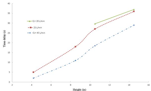
Fig. 5 Effect of spray nozzle heights on the delay of wetting start for various spray flow rates
