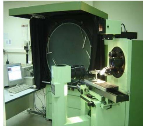
(a) Test set up for Profile Projector
