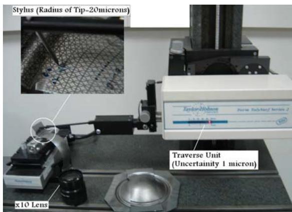
Fig. 5 Measurement of circle diameters by Form Talysurf
