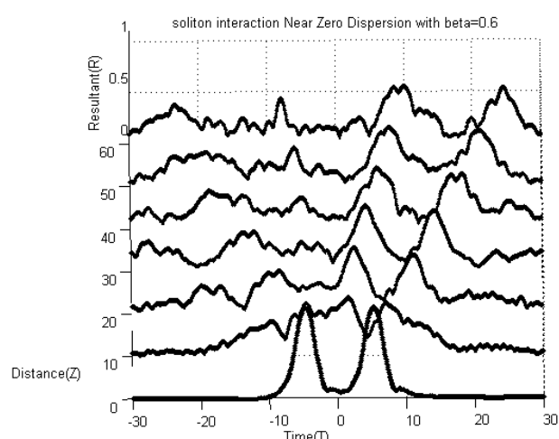
Fig. 15(b) 3-Dimensional plot for interaction between the adjacent soliton pulses at zero-dispersion wavelength with \beta=0.6 after 40 soliton periods ( Z=20\pi ).
