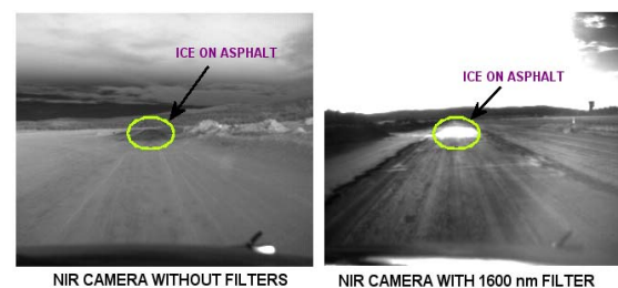
Fig. 7 Ice on road detection with utilising near infrared band
