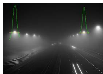
Fig. 10 The halo around artificial light sources under night-time fog conditions can be used to detect night fog
