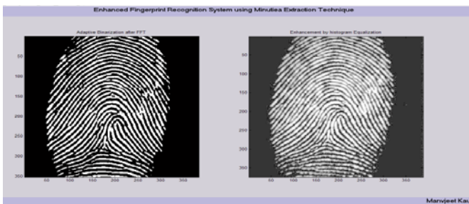
Fig. 8 the Fingerprint image after adaptive binarization Binarized image (left), Enhanced gray image (right)
