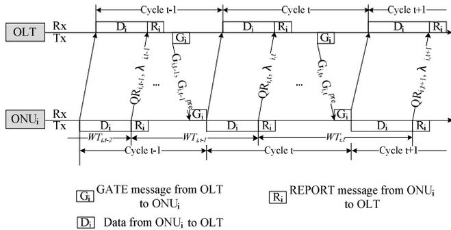
Fig. 3 Timing diagram of ASPQR
