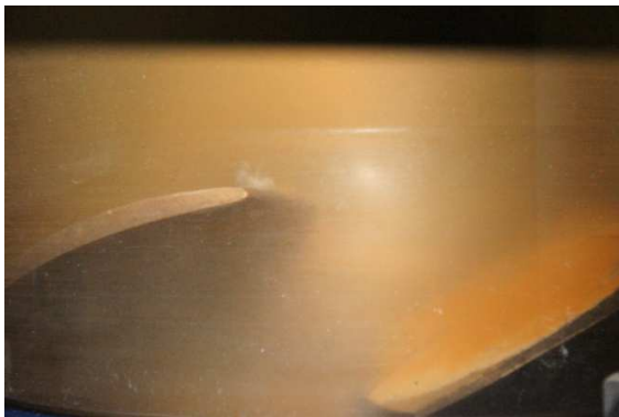
Fig. 9 Cavitation pattern under operating condition of No. 2-4
