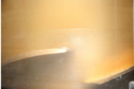
Fig. 4 Cavitation pattern under operating condition of No. 1-4
