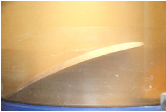
Fig. 7 Cavitation pattern under operating condition of No. 2-2
