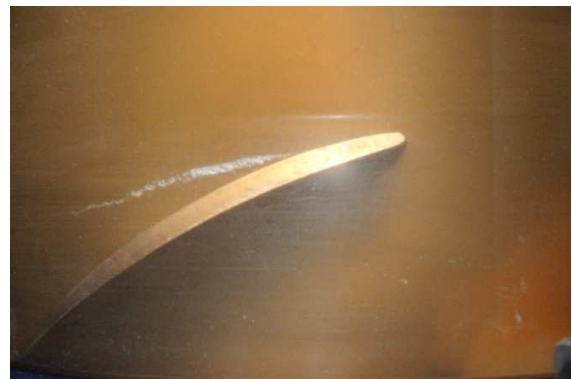
Fig. 11 Cavitation pattern under operating condition of No. 3-1
