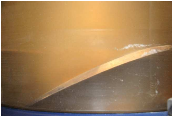
Fig. 8 Cavitation pattern under operating condition of No. 2-3
