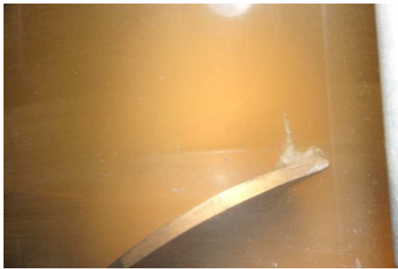
Fig. 13 Cavitation pattern under operating condition of No. 3-3
