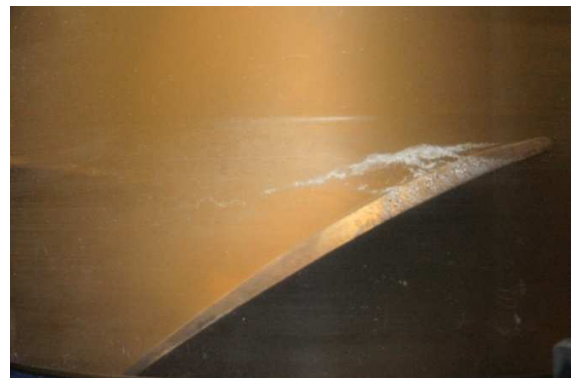
Fig. 12 Cavitation pattern under operating condition of No. 3-2
