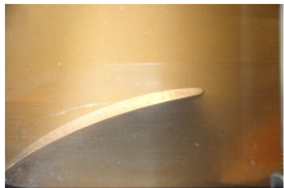
Fig. 6 Cavitation pattern under operating condition of No. 2-1
