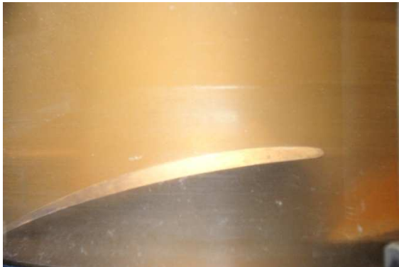
Fig. 3 Cavitation pattern under operating condition of No. 1-3
