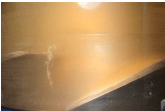
Fig. 10 Cavitation pattern under operating condition of No. 2-5
