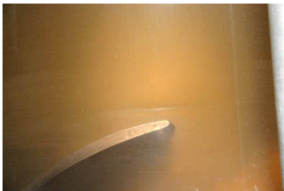
Fig. 14 Cavitation pattern under operating condition of No. 3-4
