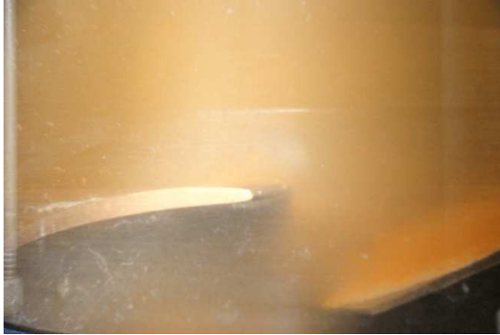
Fig. 1 Cavitation pattern under operating condition of No. 1-1
