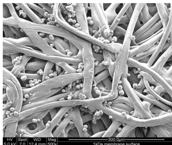
Fig. 14 SEM image of the surface of regenerated cellulose 1kDa membrane under 500 x magnifications
