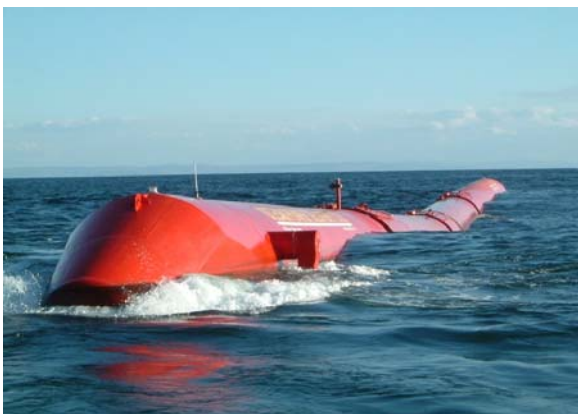
Fig. 5 Pelamis machine facing the sea waves. (From Ocean Power Delivery)
