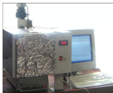
Fig. 2 Fabricated heating chamber around TPA cross head
