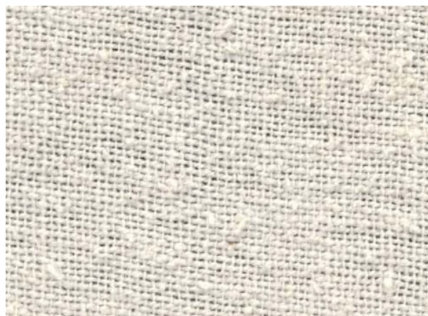
Fig. 1. Scanned surface of pilled fabric
