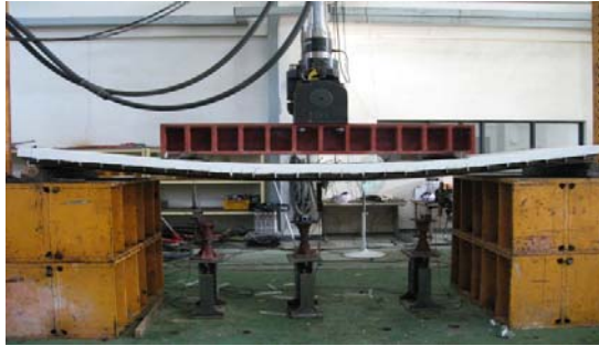
Fig. 3 Deflection under maximum loading condition
