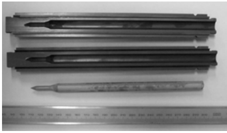
Fig. 2 Graphite mould used in this study and as-grown crystal of pure Mg
